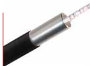
Residual dielectric and bonding compound on conductor after coring
